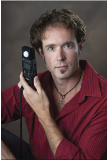
PLATE 4 —In this image of Brian Caplan, the light meter dome is pointed toward the main light source to read the amount of light illuminating the subject. The corresponding aperture or f-stop will appear on the meter's LED screen with the actual exposure of the main light source. You may need to increase or decrease the power of your strobe to obtain the desired f-stop. When working with strobes, your exposure is controlled only by your f-stop, not by your shutter speed. More on this later. (Manual mode; ISO 100; 1/250 second; f/9.0)
